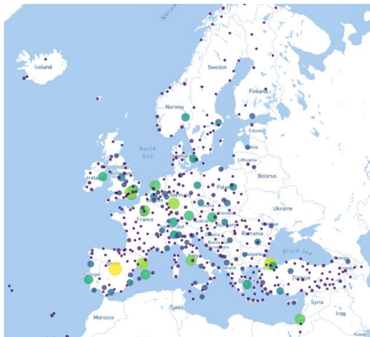
Figure 14 Energy (H 2 ) required at different Aerodromes to support the network of hydrogen flights in the Medium Range market segment
