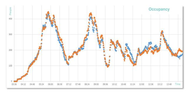
Orange curve: Occupancy based on manual in/out counts. Blue curve: Occupancy based on a Cam/WiFi Hybrid solution.
