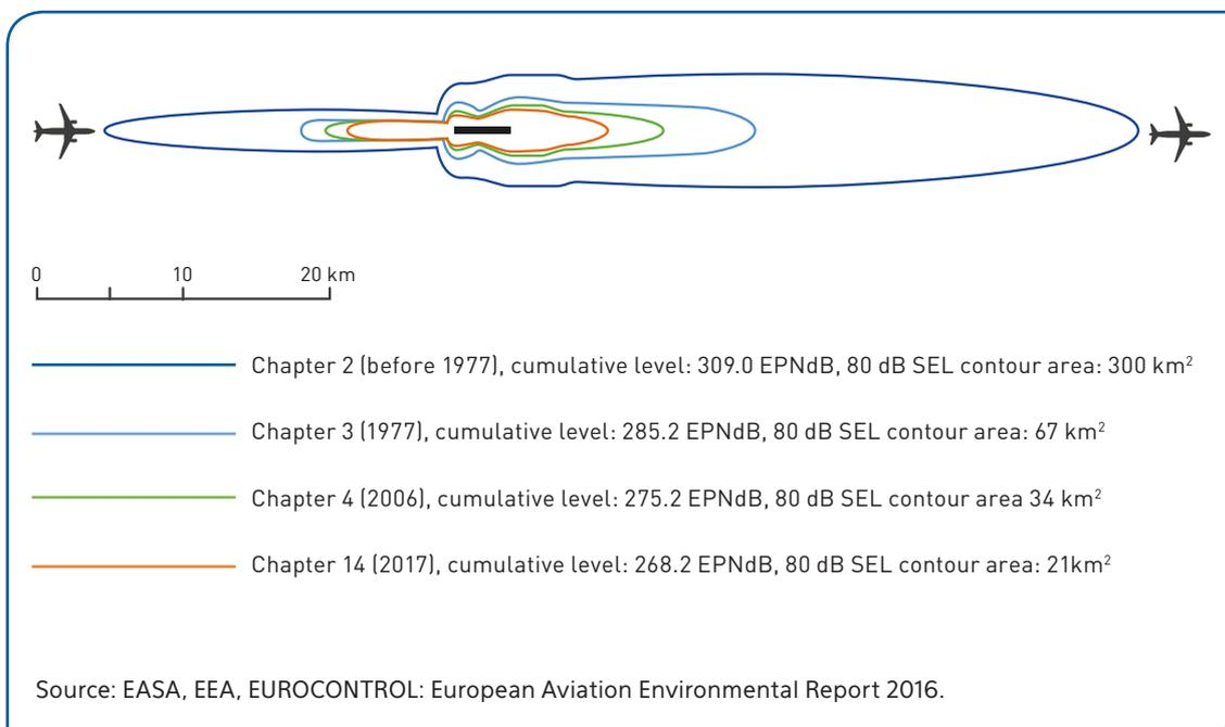
The graphic below spells out how each of the key manufacturers have advanced with reducing the noise emissions of their aircraft, in line with changes to ICAO's Chapters.
